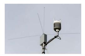
The data logger, power supply and the batteries are mounted on the mast at cca. 1,5m height.
